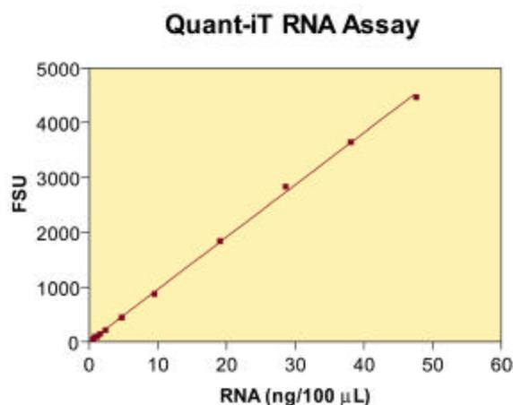
**Figure 1.** *r*RNA and Quant-iT RNA analyzed using the Modulus and the Red Fluorescence Optical Kit. 5  $\mu\text{L}$  of each standard was added to 100  $\mu\text{L}$  of Quant-iT RNA reagent. 100  $\mu\text{L}$  of this mixture was subsequently transferred to a minicell cuvette and Modulus measured under the Raw Fluorescence Mode of each dilution.
